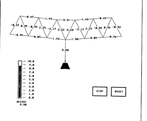
Fig. 9. Simulating a bridge under load.
